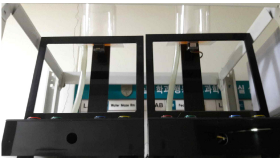
Mouse fear conditioning chamber
